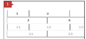
Figure 2: Begin by cutting plank 1 in half. Position the cut end of plank 1 against the wall in the left corner of the room.
